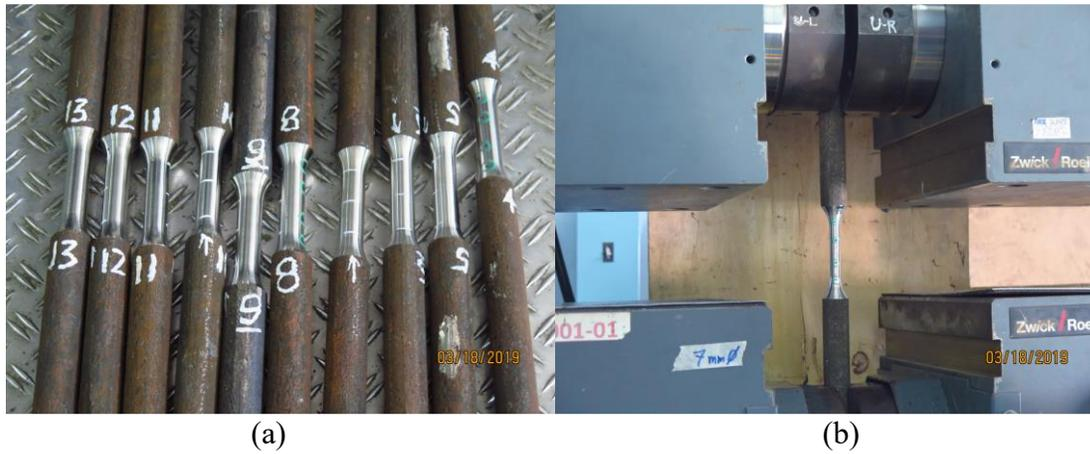
**Figure 2.** Images of (a) machined samples for tension test and (b) sample undergoing tension test
