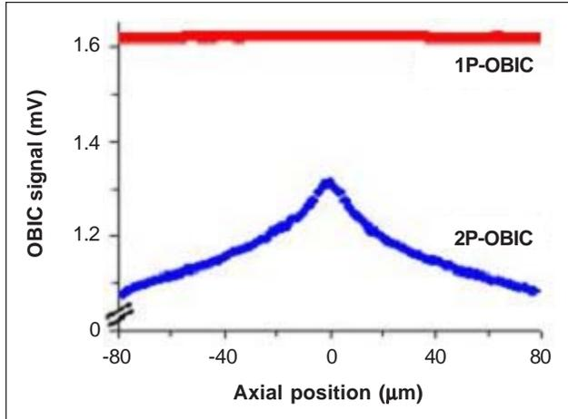
Fig. 3. Focal dependence of the generated OBIC signal. Throughout the scanned axial positions, 2P-OBIC changes while 1P-OBIC remains insensitive. The 2P-OBIC axial profile has a FWHM value of 50  $\mu\text{m}$ .
