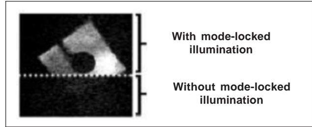
Fig. 4. 2P-OBIC imaging of LED with and without mode-locked illuminations. Image size is 625 x 625  $\mu\text{m}$ .
