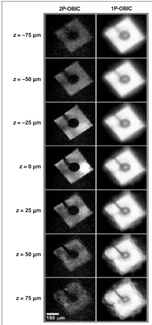
Fig. 5. Representative 2P-OBIC and 1P-OBIC images of the LED sample at different focal positions.
