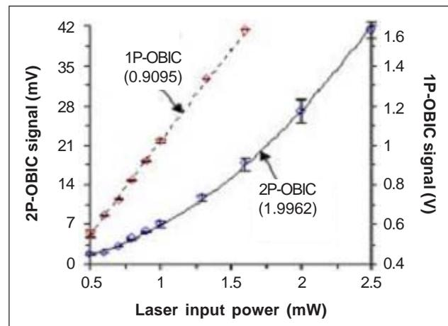
Fig. 2. Power dependence of the generated OBIC signal. The slopes of the 2P-OBIC and 1P-OBIC responses are 1.9962 and 0.9095, respectively.
