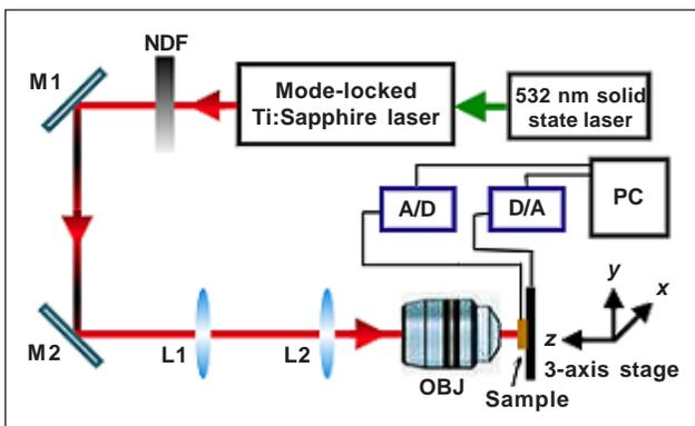
Fig. 1. Schematic diagram of the stage-scanning 2P-OBIC microscope used.
