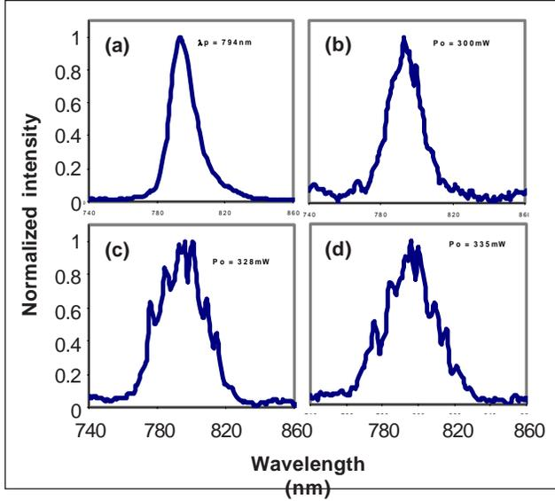
Fig. 3. Input and output spectra measured using a mochromator on a 50 cm PCF for different pump powers: (a) Input pump,  $\lambda_p = 794$  nm, (b)  $P_o = 300$  mW, (c)  $P_o = 328$  mW, and (d)  $P_o = 335$  mW.
