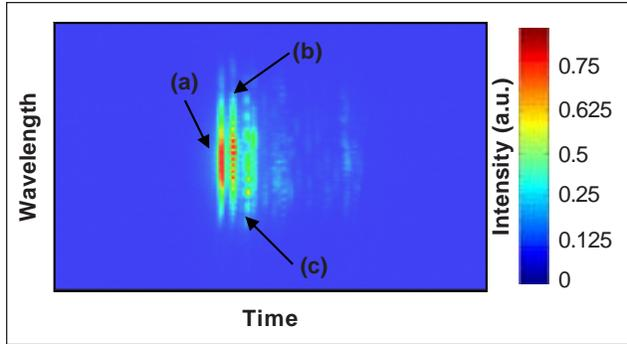
Fig. 6. Spectrogram of the output pulse reveals decomposition of the input into different modes.
