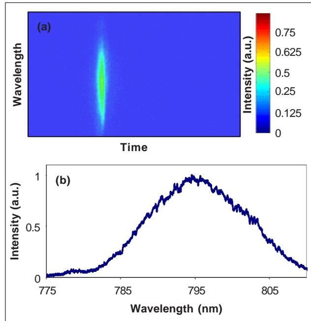
Fig. 5. (a) Spectrogram of the input pulse captured by a streak camera. (b) spectral profile of the input pulse.
