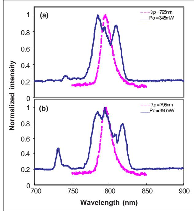
Fig. 4. Input and output spectrum measured on a 100 cm PCF pumped at 795 nm for different pump powers: (a) 345 and (b) 350 mW.
