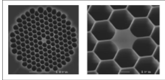
Fig. 2. Scanning electron micrograph (SEM) photos of an (a) array of air-silica cladding and (b) pure silica core in a highly nonlinear PCF. (Source: <http://www.blazephotonics.com>)
