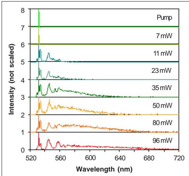
Fig. 3. Output spectra of the 51-m-long single-mode fiber for different pump powers.
