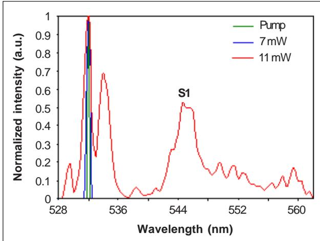
Fig. 2. Spectrum on the fiber output featuring the evolution of the 532 nm laser pulse towards the first-order Stokes S1 and generation of spectral sidebands with increasing power.
