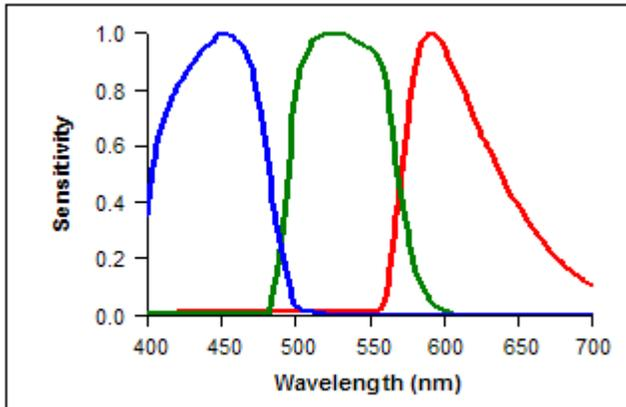
Fig. 1. Camera sensitivities of 3CCD camera with null filter.
