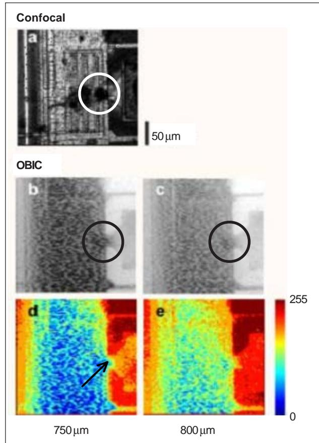
Fig. 4. (a) Confocal and (b) OBIC images of an integrated circuit with an electrical overstress defect (encircled region). The OBIC images are taken using 750 and 800 nm. (c) False color images of the OBIC reveal nonuniform generation of OBIC near the defect area. Arrow indicates a disruption of OBIC that could be due to the defect.
