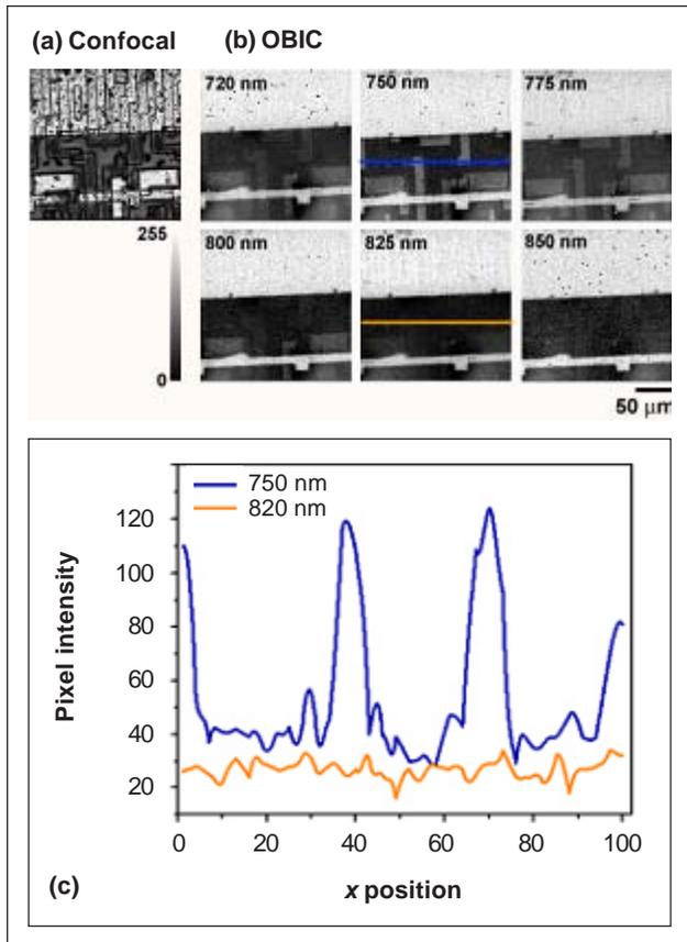
Fig. 2. (a) Confocal and (b) OBIC images of a photodiode array. The confocal image was acquired at the focus of the system using 750 nm. The OBIC images shown are taken using different illumination wavelengths (720, 750, 775, 800, 825, 850 nm). (c) Line scans of the images reveal structures that appear on certain wavelengths (750 nm) which are previously absent on others (825 nm).
