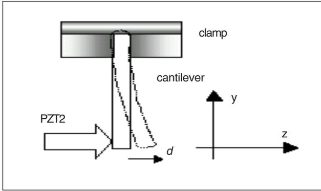
Fig. 3. Cantilever and displacement,  $d$ .
