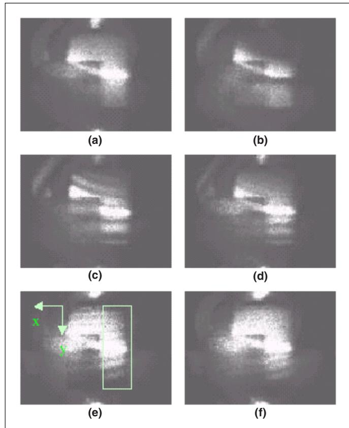
Fig. 4. (a) Reconstructed object without deformation. Holographic interferograms obtained for a voltage difference of (b) 10 V, (c) 30 V, (d) 35 V, (e) 40 V, and (f) 50 V.
