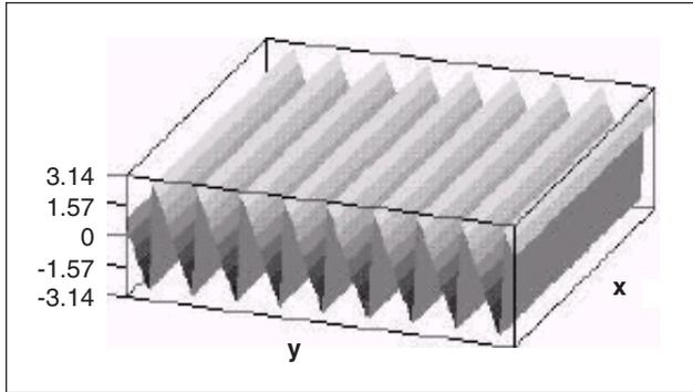
Fig. 5. Phase distribution (wrapped in  $2\pi$ ) obtained after applying the FTM (Fourier transform method) on the rectangular region in Fig. 4 e.
