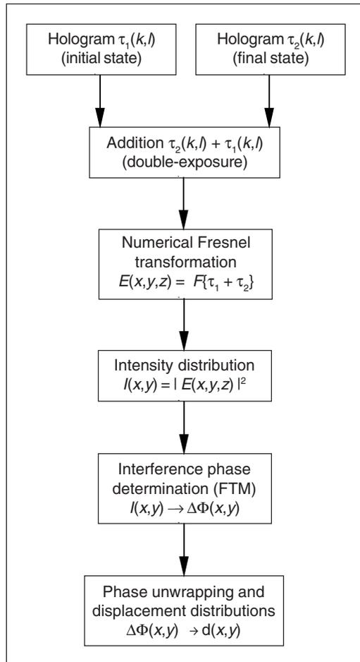
Fig. 1. Digital holographic interferometry for measurement of out-of-plane displacements.
