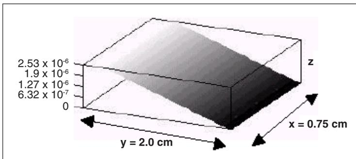
Fig. 6. 3D plot of the surface deformation for a voltage difference of 40 V ( $z$ -axis is in meter).
