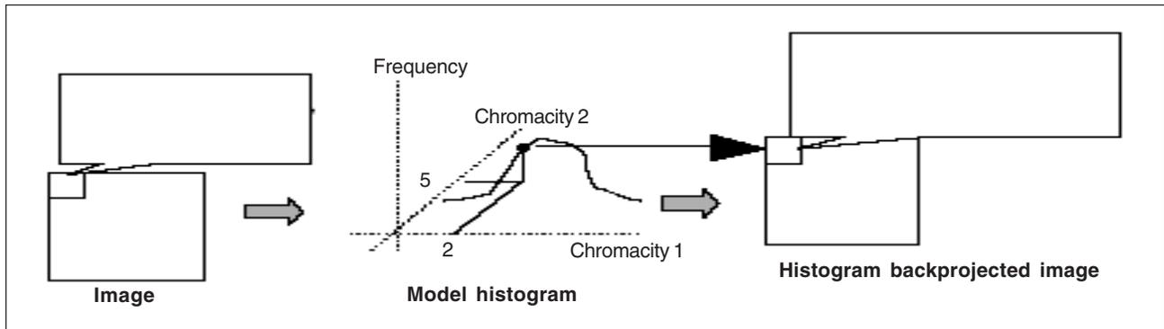
Fig. 1. Illustration of the Histogram Backprojection technique. The chromaticity values of a pixel are traced into the color histogram of a query image and its frequency value is assigned to that pixel.
