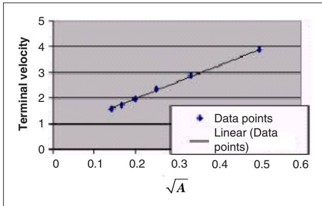
Fig. 4. Graph of  $v$  versus  $\sqrt{A}$ .
