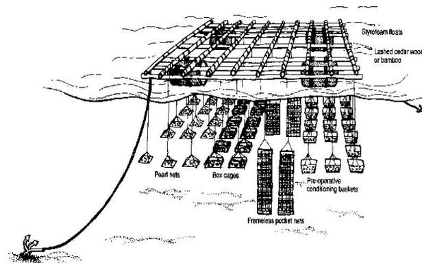
Figure 5. Alternative method for farming oysters on rafts in deep water. Raft pearl farm structure from Gervis & Sims 1992.
