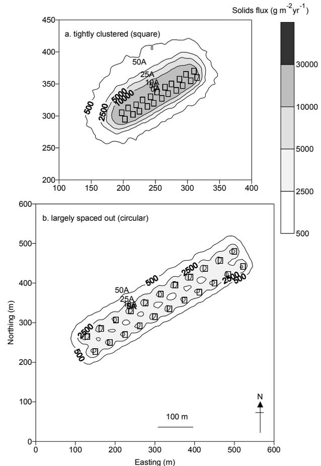
Figure 1. Model predictions of flux ( $\text{g m}^{-2} \text{yr}^{-1}$ ) showing the significant difference in deposition footprint severity and extent when tightly clustered square cages (a) are replaced by circular cages spaced 30m (b). For the spaced-out cages, areas of lower flux are shown in between lines of cages which will tend to assist sediment processes (MERAMED, <http://meramed.akvaplan.com>).
