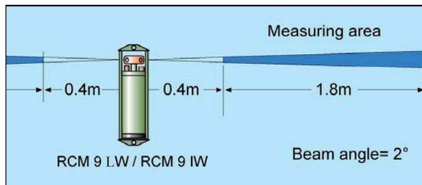
Figure 1. Illustration of the measuring area for the RCM 9 LW current meter
