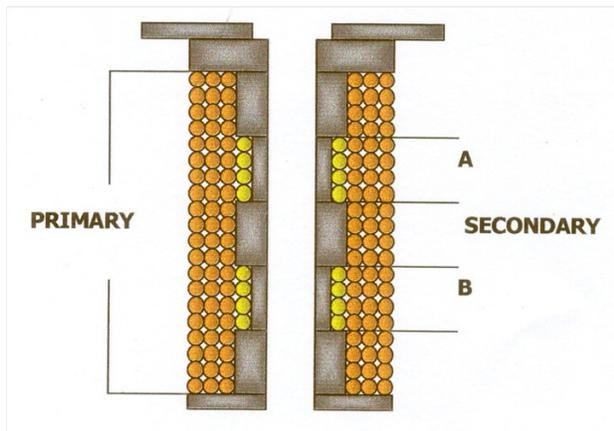
**Figure 1.** Hartshorn-type Mutual Inductance Bridge. An alternating current creates an alternating magnetic field through the primary coil, which induces emf across the two secondary pick-up coils A and B.
