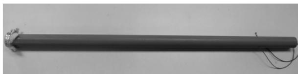
Figure 13. Pore water pressure sensor
