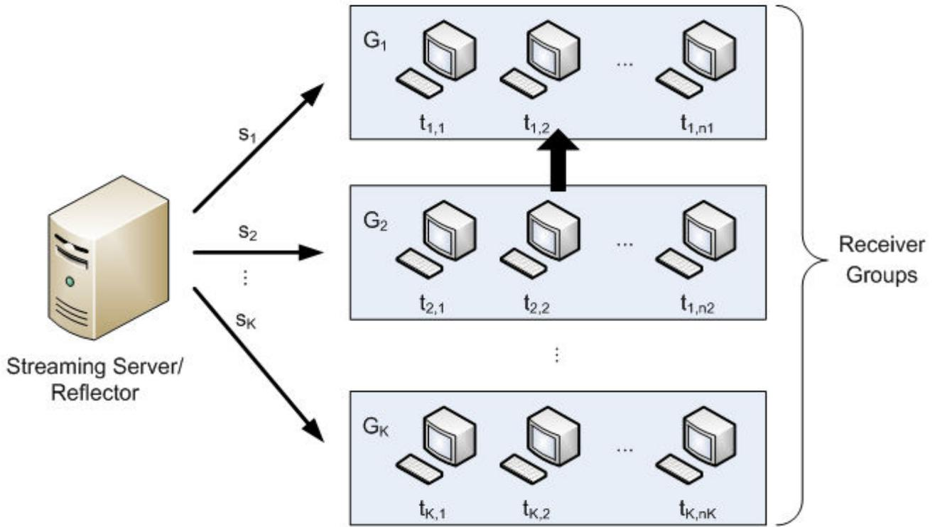
Figure 1. Terminal grouping according to the received stream bitrate.
