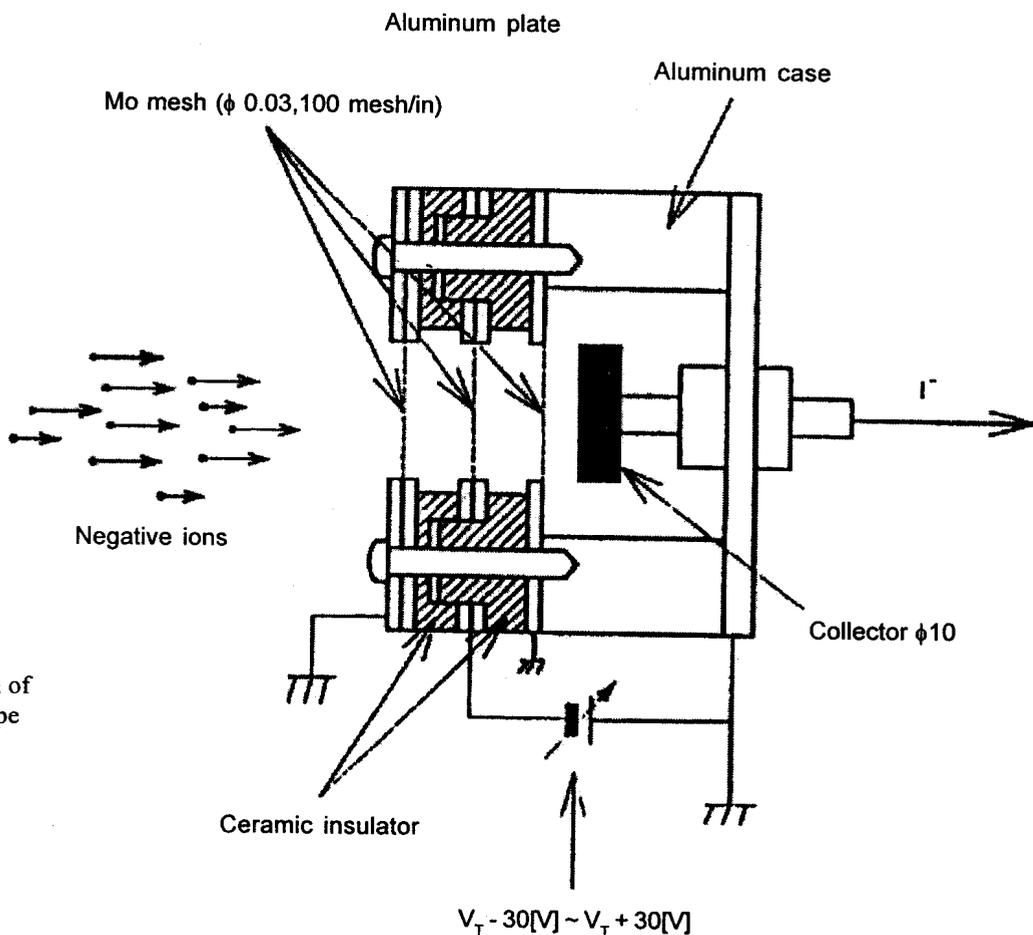
Fig. 3. Schematic diagram of the retarding potential-type energy analyzer.
