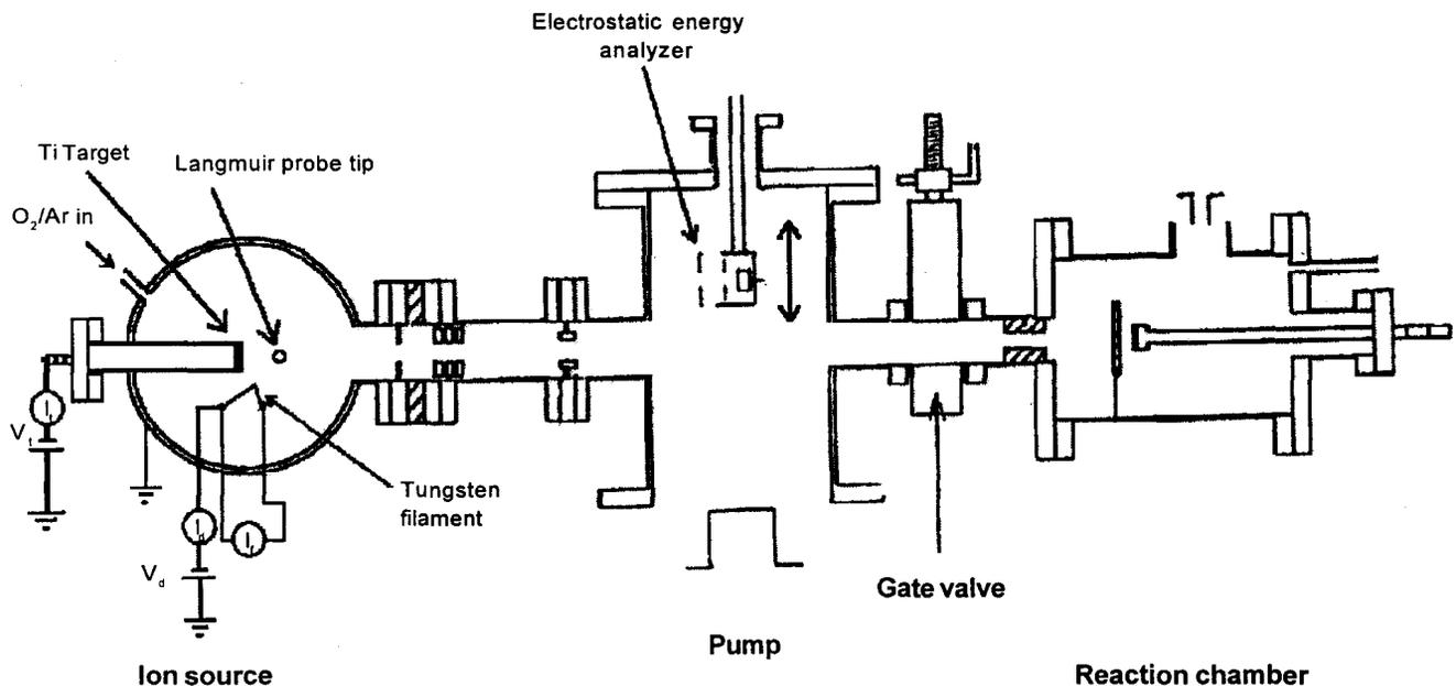
Fig. 1. Schematic diagram of the experimental set-up. The Langmuir probe is found inside the ion production chamber while the ESA is located inside the connecting chamber.
