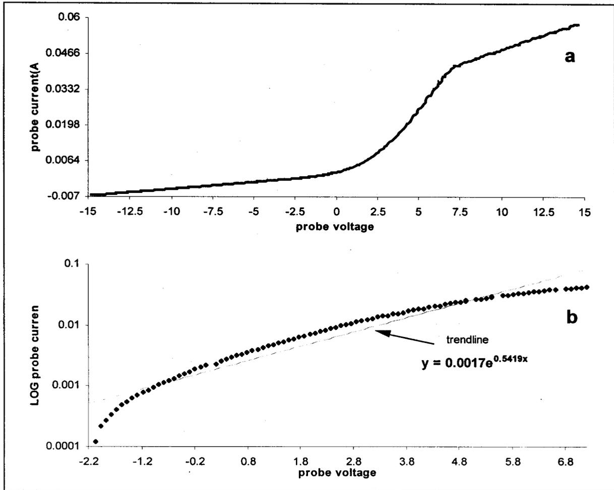
Fig. 4(a). Averaged Langmuir trace; (b) Log plot of the transition region. Operating parameters for the discharge are discharge current = -0.8A, discharge voltage = -40V, target voltage = -200V, target current = -30 mA and filament current = 8.5A.
