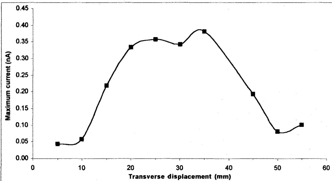
Fig. 6. Plot of maximum ESA current for different transverse displacements. Operating parameters for the discharge are discharge current =  $-0.8\text{A}$ , discharge voltage =  $-40\text{V}$ , target voltage =  $-200\text{V}$ , target current =  $-30\text{mA}$ , and filament current =  $8.5\text{A}$ .
