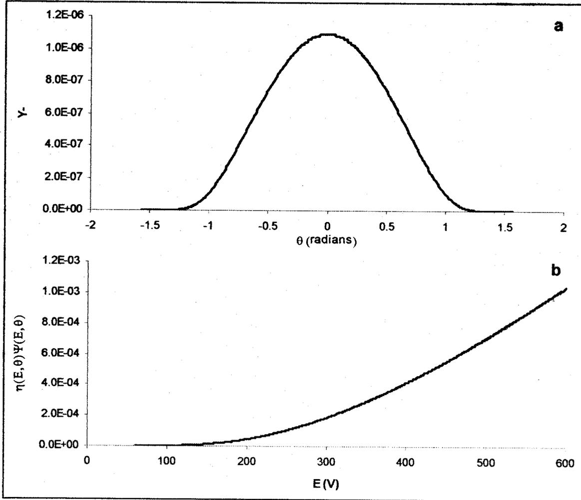
Fig. 7. (a) Plot of the energy distribution  $Y$  as a function of the ejection angle ( $-\pi/2 \leq \theta \leq \pi/2$ ) for  $E=200$  V. This gaussian curve concentrates most of the ions near the propagation axis of the chamber but broadens with propagation. (b) Plot of the  $h(E, \theta)\Psi(E, \theta)$  as a function of  $E$ .
