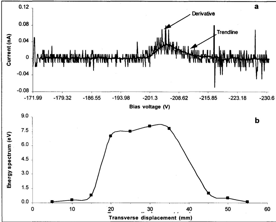
Fig. 8. (a) Representative plot of the derivative of the ESA trace for  $x = 35$  cm. The solid line is the trendline obtained by the moving average protocol. (b) The FWHM of the energy spectrum for different  $x$  values. Operating parameters for the discharge are discharge current = -0.8A, discharge voltage = -40V, target voltage = -200V, target current = -30 mA and filament current = 8.5A.
