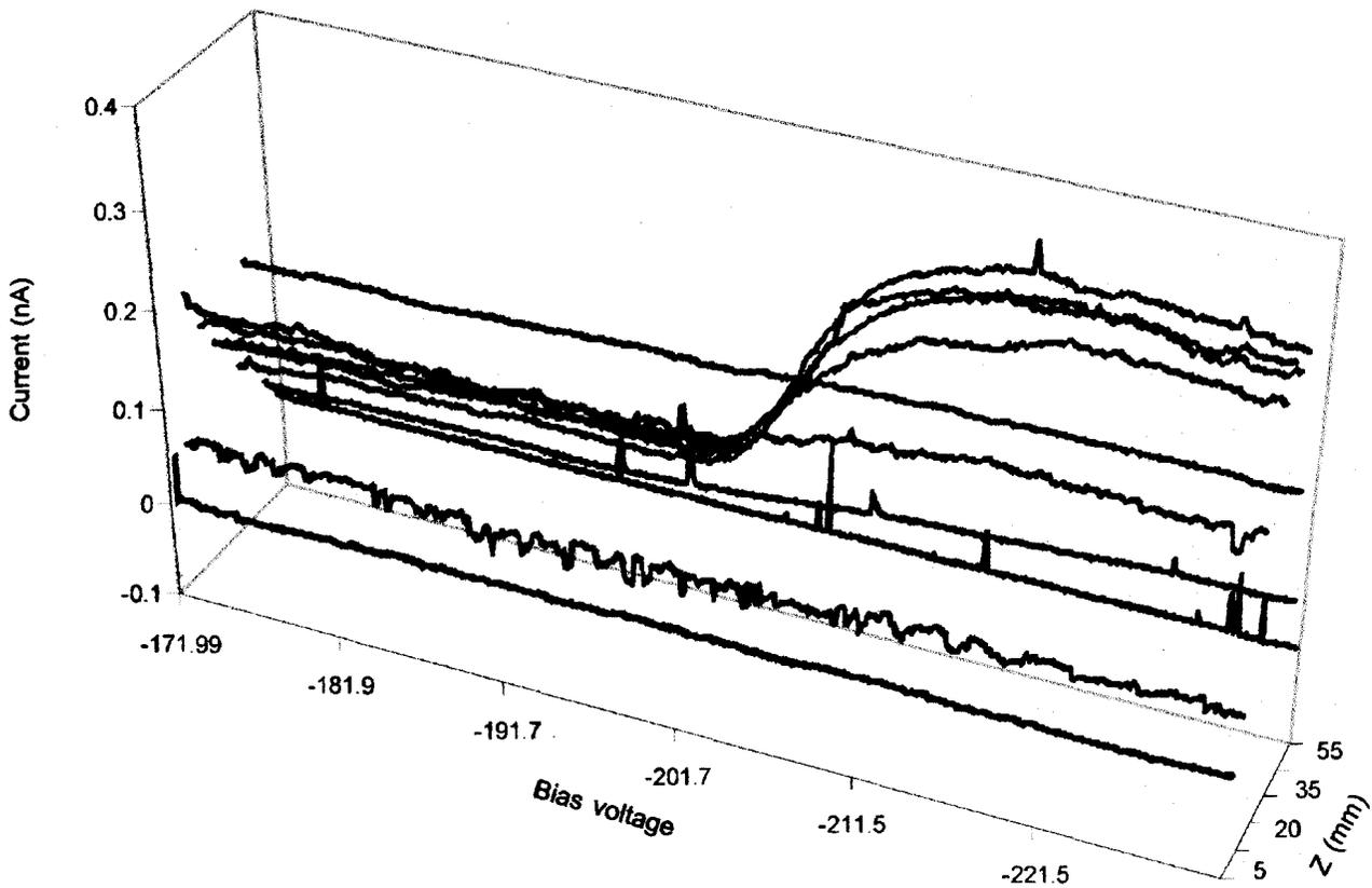
Fig. 5. ESA traces for different longitudinal displacements  $Z$ . Operating parameters for the discharge are discharge current =  $-0.8\text{A}$ , discharge voltage =  $-40\text{V}$ , target voltage =  $-200\text{V}$ , target current =  $-30\text{mA}$ , and filament current =  $8.5\text{A}$ .
