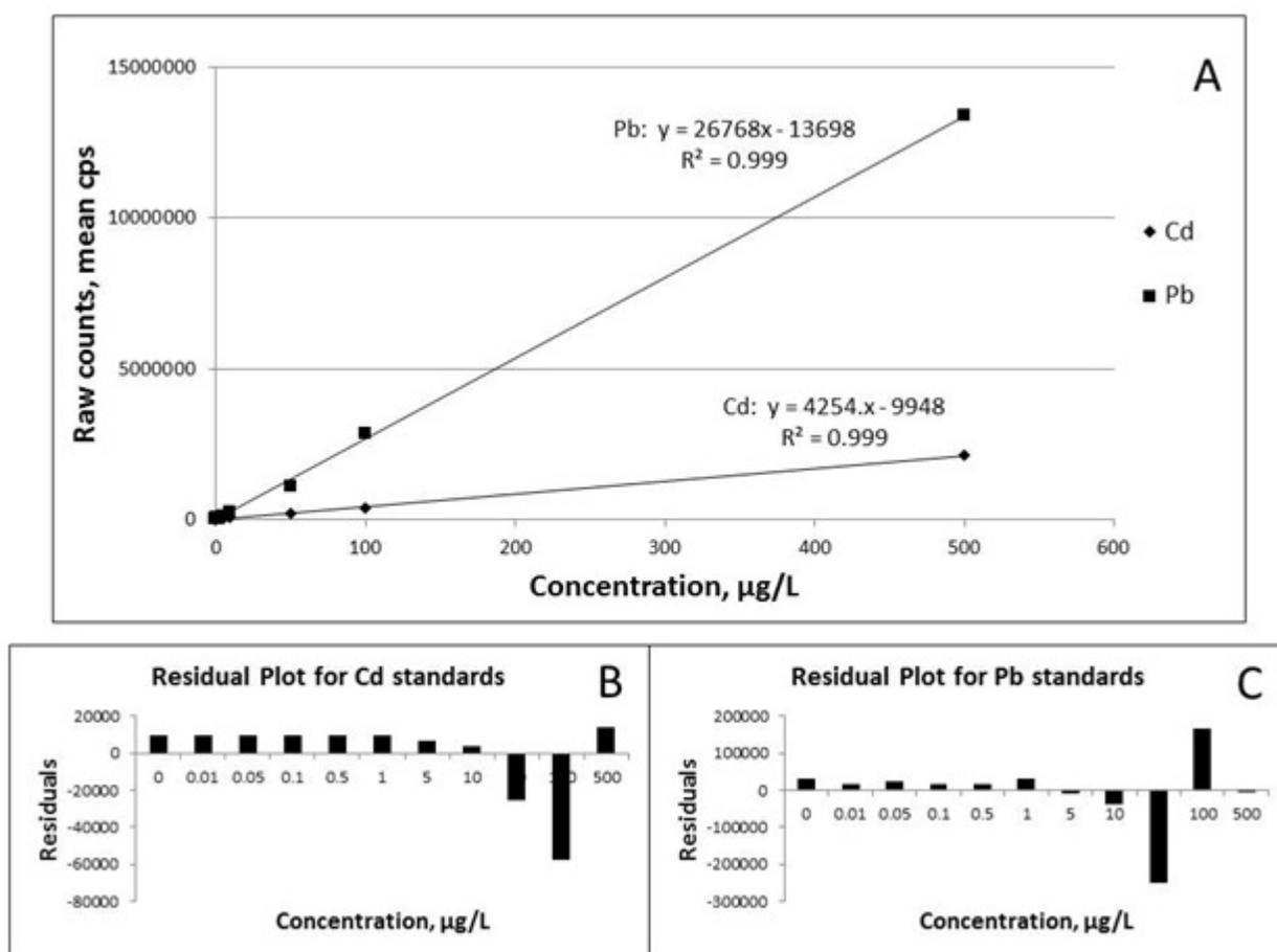
Figure 2. Evaluation of the linearity of the calibration standard solutions. (2A) shows the linearity of the calibrations standard solutions; (2B) and (2C) show results of the residual analyses for Cd and Pb standard solutions, respectively.
