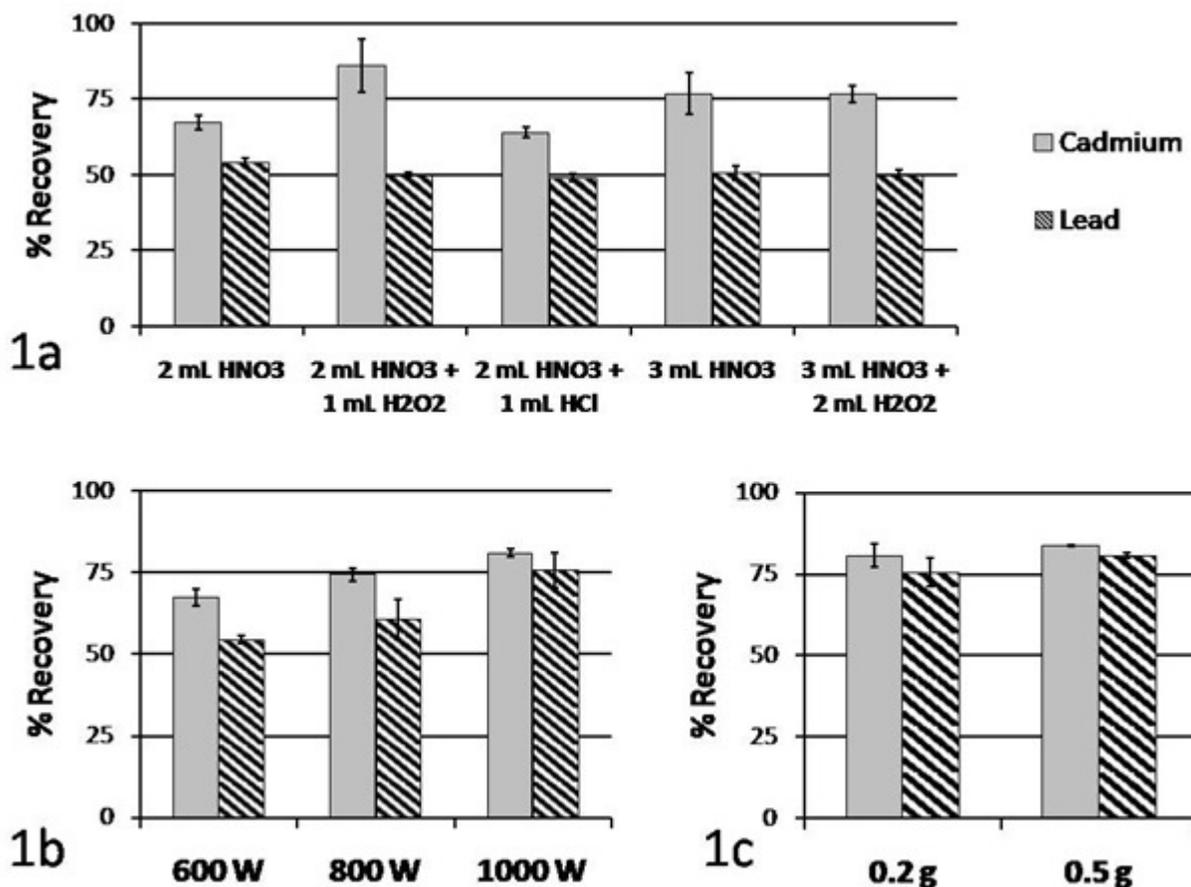
Figure 1. Percent recoveries of Cd and Pb as a function of different digestion parameters (acid used in the digestion, maximum power and amount of sample): (1a) effect of the use of different acid, acid mixtures, and mixture of acid and oxidizing agent on the percent recovery of the analytes in the reference material (amount of sample: 0.2 g; power: 600 W; digestion period: 45 min); (1b) effect of the maximum power used in digestion and (1c) effect of the amount of sample digested
