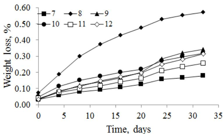
Figure 2. Migration kinetic curves of additives in rubber compounds 7–12
