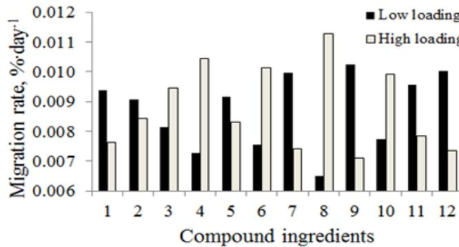
Figure 5. Effect of ingredient loading on surface migration rate of additives.
