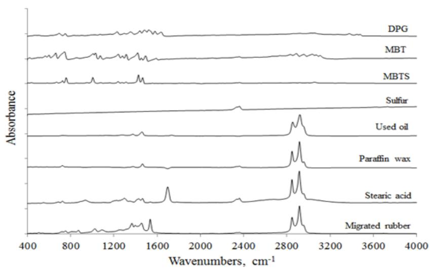
Figure 13. ATR-FTIR spectra of sample migrated and cleaned rubber specimen, raw natural rubber, and compounding ingredients 6-12.
