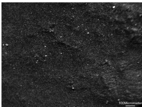
Figure 14. Additive blooming in compound 14 at ambient conditions.
