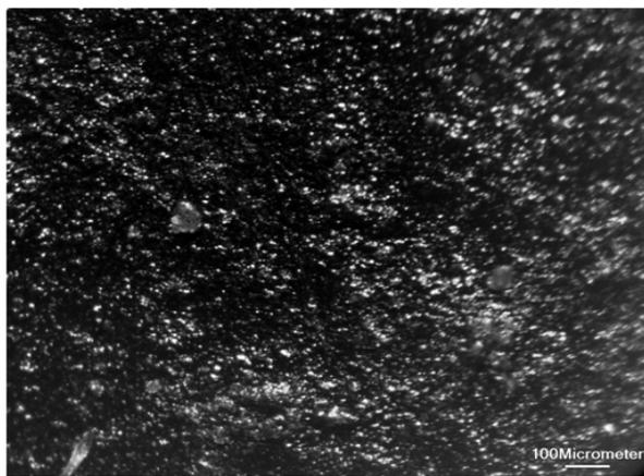
Figure 16. Additive bleeding in compound 12 at ambient conditions.
