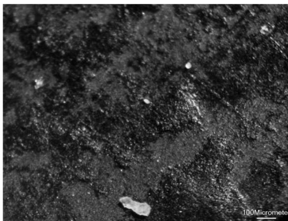
Figure 15. Additive blooming in compound 16 at ambient conditions.
