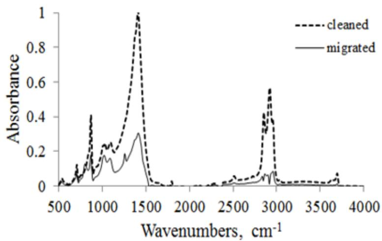
Figure 11. ATR-FTIR spectra of cleaned and migrated rubber surfaces of compound 15.
