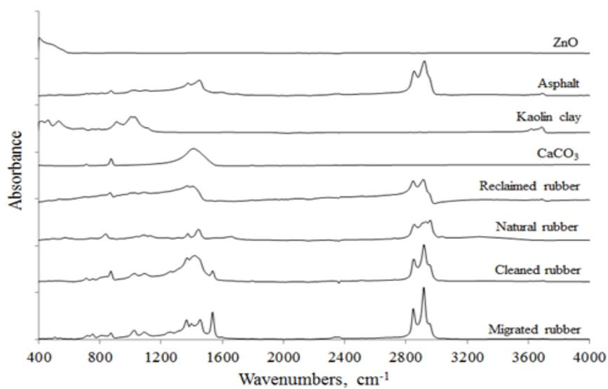
Figure 12. ATR-FTIR spectra of sample migrated and cleaned rubber specimen, raw natural rubber, and compounding ingredients 1-5.
