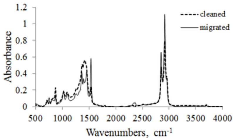
Figure 10. ATR-FTIR spectra of cleaned and migrated rubber surfaces of compound 1.
