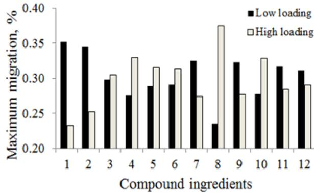
Figure 4. Effect of ingredient loading on maximum amount of additive migration.
