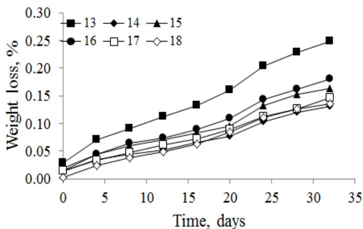
Figure 3. Migration kinetic curves of additives in rubber compounds 13–18
