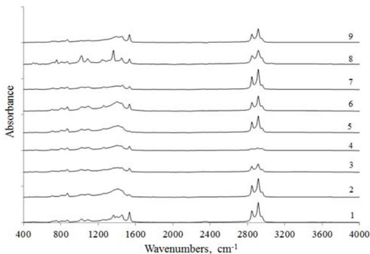
Figure 8. ATR-FTIR spectra of migrated rubber surfaces for compounds 1–9.
