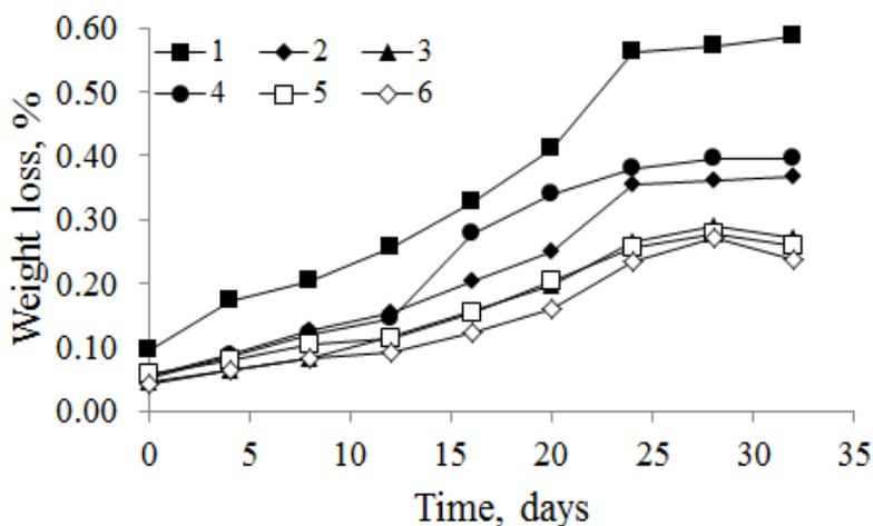
Figure 1. Migration kinetic curves of additives in rubber compounds 1–6.
