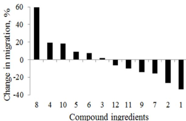
Figure 6. Ranking of compounding ingredients in terms of their effect on maximum amount of additive migration.
