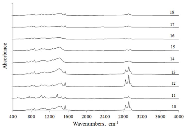
Figure 9. ATR-FTIR spectra of migrated rubber surfaces for compounds 10–18.
