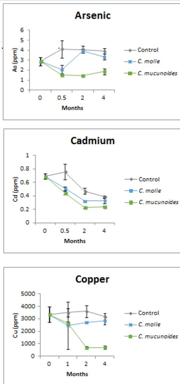
Figure 3. Reduction of As, Cd, and Cu concentrations in mine tailings before and after the experiment. Values indicate Mean  $\pm$  SE; n = 3; in parts per million.
