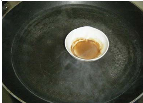
Figure 1. Hot Water bath set-up for the evaporation of moisture.
