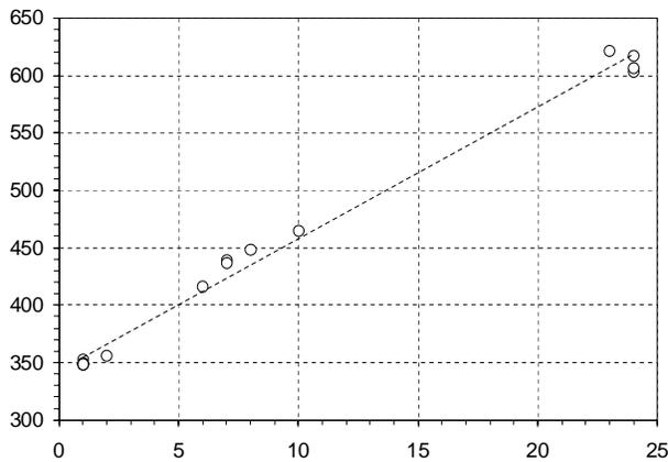
Figure 12. Multiplication completion times (ordinary cases) in ns as a function of the number of 1's in  $FX$
