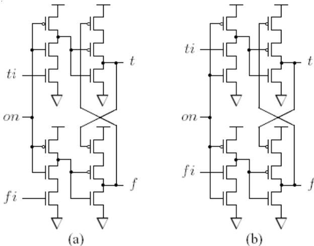
Figure 3. Transistor-level schematics of (a) decide early, (b) decide late
