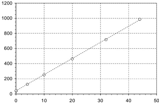
Figure 16. Remainder completion times ( $X = Y$ ) in ns as a function of the number of shifts to normalize operands
