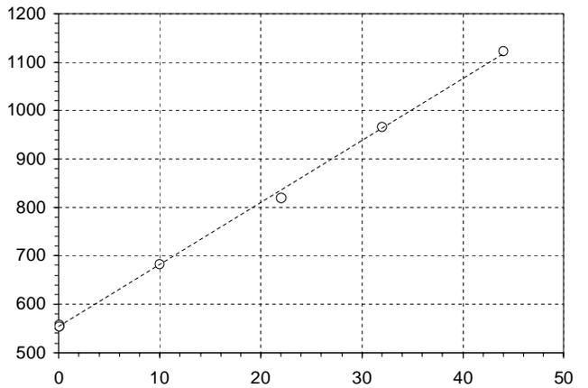
Figure 14. Division completion times (ordinary cases, with one 1 in  $Fz'$ ) in ns as a function of the number of shifts to normalize operands
