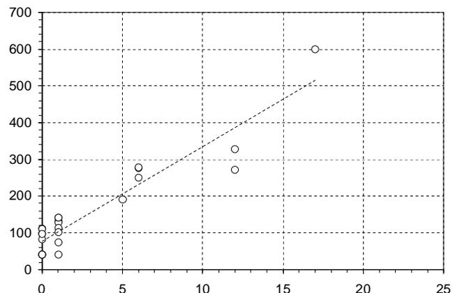
Figure 15. Remainder completion times (ordinary cases, w/o denormal operands,  $eX \geq eY$ ) in ns as a function of  $z$
