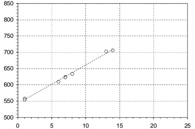
Figure 13. Division completion times (ordinary cases, without denormal operands) in ns as a function of the number of 1's in  $Fz'$
