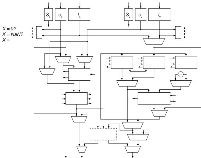
Figure 1. Block diagram of the datapath
