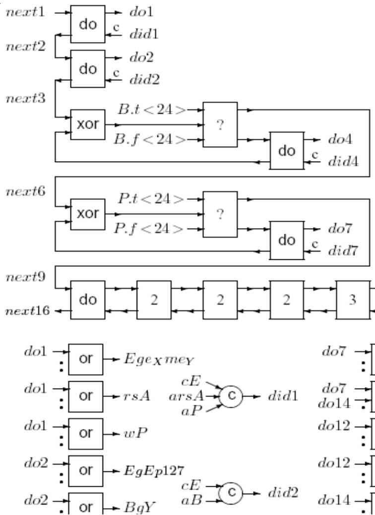
Figure 10. Implementation of sample algorithm
