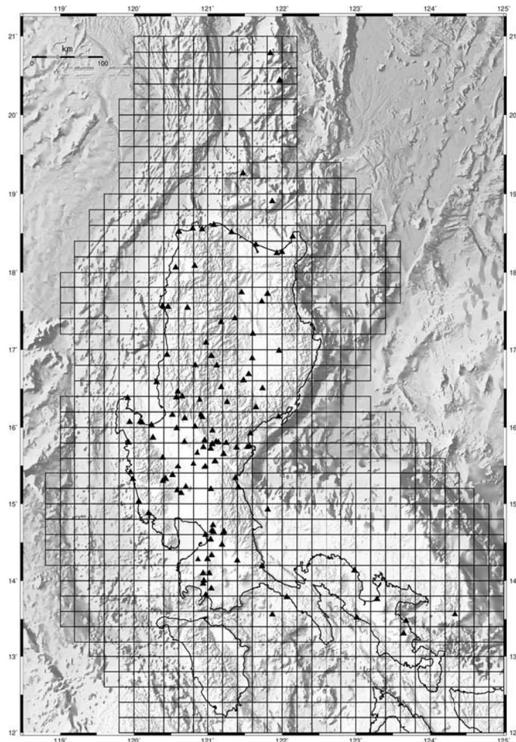
**Figure 6.** Map showing the extents of the Luzon Continuum Model. Strain rates from input block model station velocity residuals are computed within each  $0.2^\circ \times 0.2^\circ$  gridded box. The modeled region has a total of 888 gridded boxes (black lines) and contains 152 measurements or model residuals from GNSS station locations (solid black triangles). Background shows hillshaded surface topography and bathymetry in grayscale.
