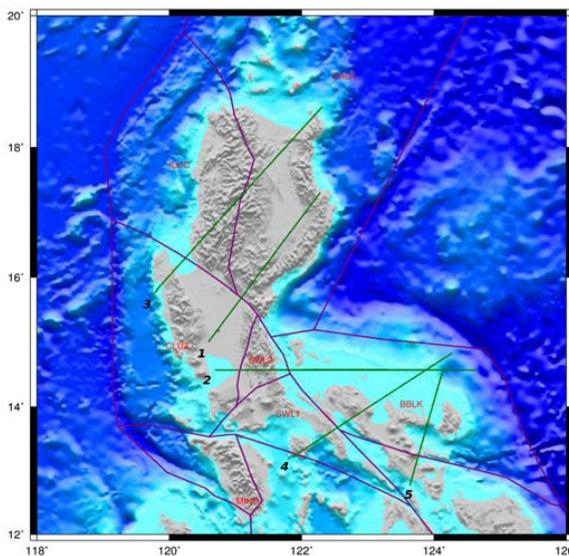
**Supplementary Figure 2.** Map of profile lines. Plots of profile lines across faults from where the model information and GPS data were obtained. Number marks the starting end of each profile line. Data were included at offset distances from either side of the profile line (i.e., 50 km Profile 1 and 100 km for Profiles 2 to 5).
