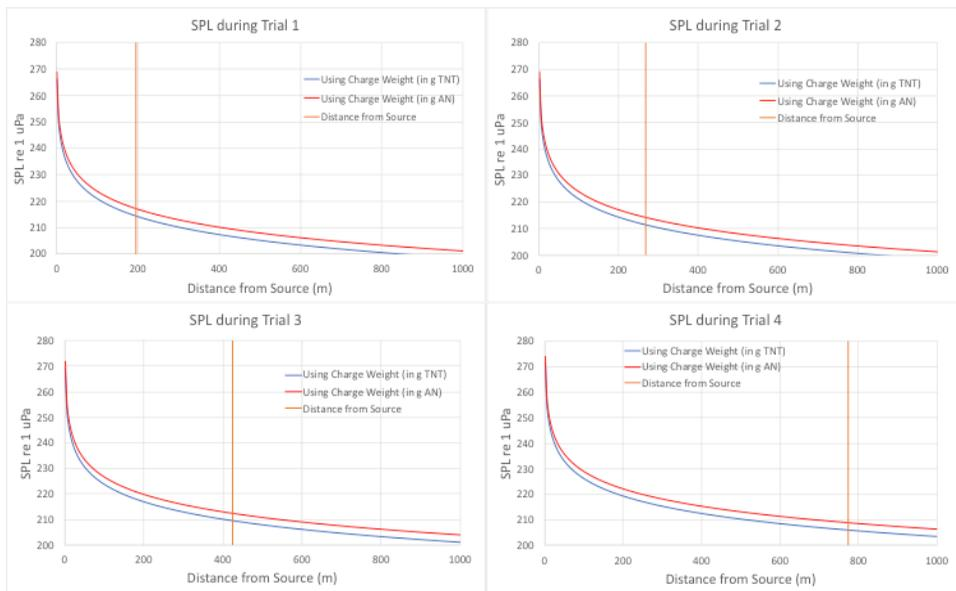
**Figure 5.** Theoretical sound pressure levels based on estimated charge weight. Orange lines indicate the distance between the source of explosion and the hydrophone setup.
