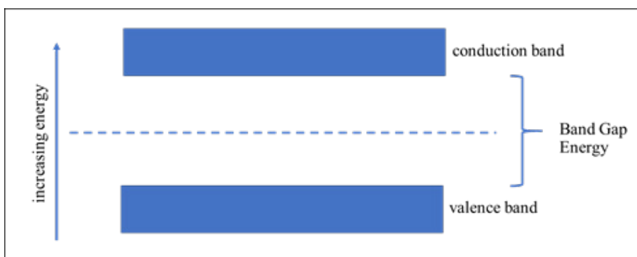
Figure 2. The band gap diagram shows the position of the valence and conduction bands. Depending on the distance or E_g , a material can be conducting or non-conducting. (Figure illustrated by Mona B. Antivola.)
