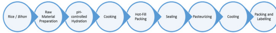
Figure 3. Production process for the preparation of acid-pasteurized RTE bihon and rice as emergency relief foods for Yolanda survivors.
